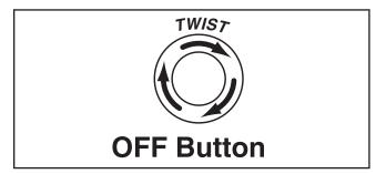
Figure 9. Resetting the switch.
